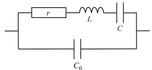
**réponses :** 1)  $\omega_r = \frac{1}{\sqrt{LC}}$  et  $\omega_a = \frac{1}{\sqrt{LC}} \sqrt{1 + \frac{C}{C_0}}$
