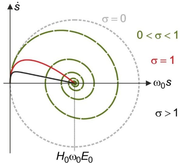
$$s_g(t) = s(t) - H_0 E_0 = A e^{-\sigma \omega_0 t} \cos(\Omega t + \psi)$$
