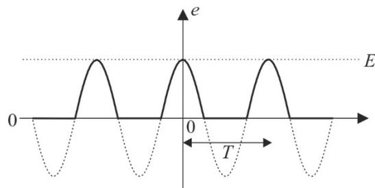
**réponses :** 1)  $e(t) = \alpha E + 2\alpha E \sum_{n=1}^{\infty} \text{sinc}(n\pi\alpha) \cos(n\Omega t)$  2)  $e(t) = \frac{E}{2} + \frac{E}{\pi} \sum_{n=1}^{\infty} \frac{\sin[n\Omega t]}{n}$
