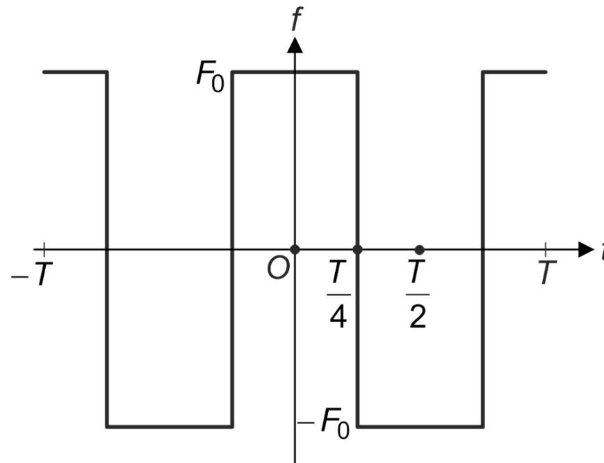
$$f(t) = \frac{4F_0}{\pi} \left[ \cos(\Omega t) - \frac{1}{3} \cos(3\Omega t) + \frac{1}{5} \cos(5\Omega t) - \frac{1}{7} \cos(7\Omega t) + \dots \right]$$
