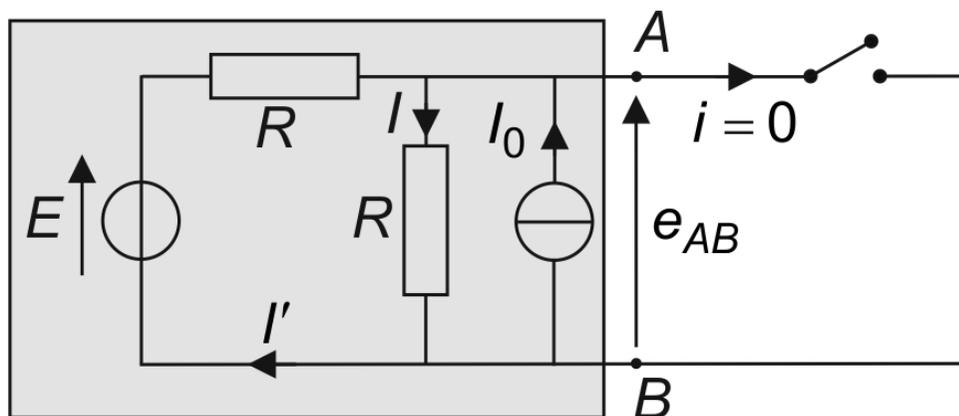
$$\left\{ \begin{array}{l} e_{AB} = RI \Leftrightarrow I = \frac{e_{AB}}{R} \\ I' = I - I_0 = \frac{e_{AB}}{R} - I_0 \\ e_{AB} = E - RI' = E - e_{AB} + RI_0 \end{array} \right.$$
