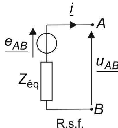
$$\underline{u}_{AB} = -\underline{Z}_{\text{éq}}\underline{i} + \underline{e}_{AB}$$
