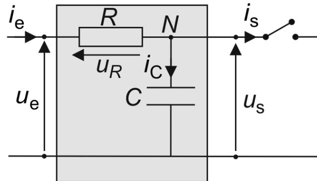
diviseur de tension  $H(j\omega) = \frac{u_s}{u_e} = \frac{\frac{1}{jC\omega}}{\frac{1}{jC\omega} + R} = \frac{1}{1 + jRC\omega}$
