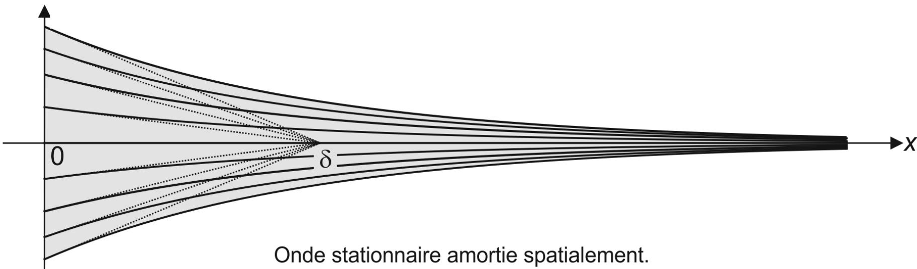
si onde  $x \nearrow$  :  $k'(\omega) > 0$  et  $k''(\omega) = +\frac{1}{\delta(\omega)} > 0 \Rightarrow \underline{s}(x, t) = s_0 e^{\frac{x}{\delta}} e^{i(\omega t - k' x)}$
